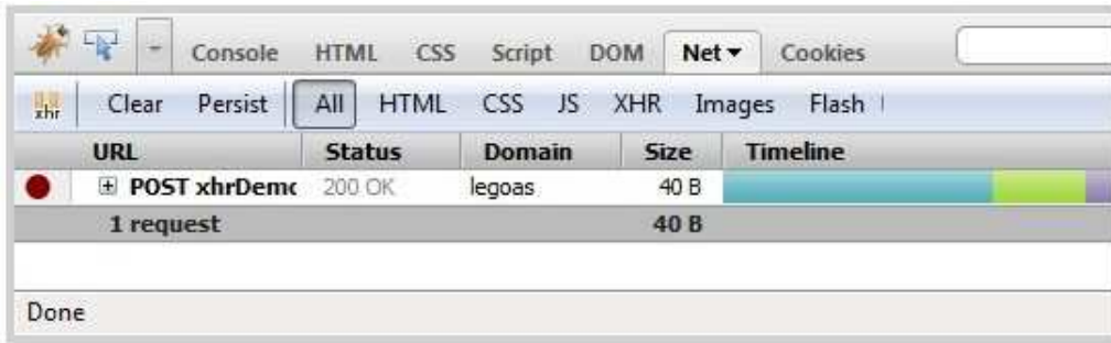
Figure 6: Setting a XHR breakpoint in the Firebug Net panel view. The developer locates the XHR request they wish to break on, and clicks in the left column. The red dot gives the user feedback that the breakpoint is set.
