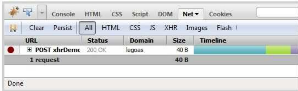
Figure 6: Setting a XHR breakpoint in the Firebug Net panel view. The developer locates the XHR request they wish to break on, and clicks in the left column. The red dot gives the user feedback that the breakpoint is set.
