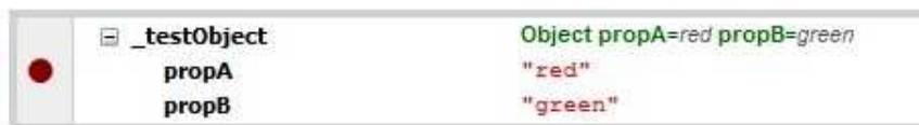
Figure 11: Part of the Firebug DOM panel, showing a breakpoint set on a property of an object.
