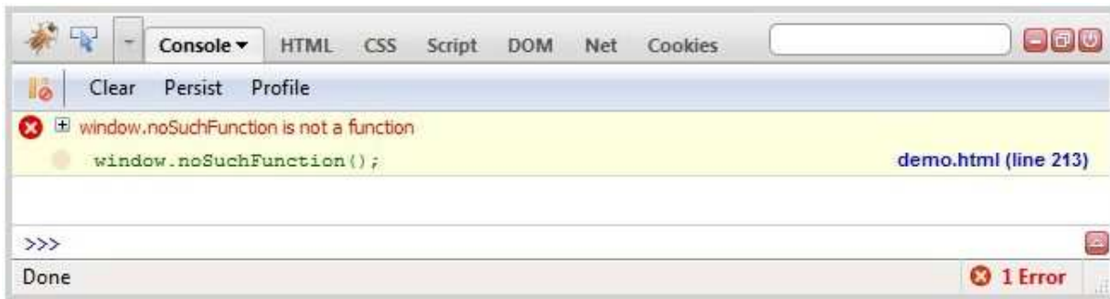
Figure 4: Part of Firebug's Console panel when an error has occurred in the Web page. The small plus sign to left of the error message opens the UI to show the call stack. Developers click on the faded red circle to set a breakpoint on the line of the error. The circle will turn dark red. Also note the orange parallel bars ("pause") button used to arm the break-on-next feature.
